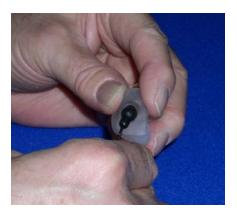
5. When observing the mold from the side you should see the CEP housing seated at the bottom of the excavation through the translucent material. The small wire exit strain relief should be positioned near the surface of the mold.
