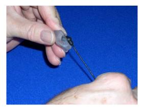
6. Fitting of the custom mold into the ear should be completed in accordance with instructions provided. The wire exit direction is a user preference and may take some experimentation. The wire may loop over the ear as shown below or a simple exit downward under the ear seal.
