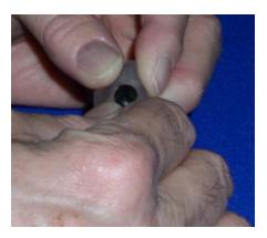
4. As the CEP is forced into the excavation, rotate the housing so that the wire exit point is adjacent to the flat surface of the custom mold.
